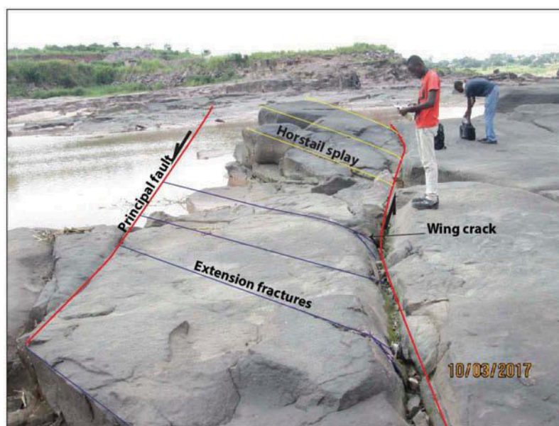
Figure 13. Strike-slip fault showing both a wall damage zone with extension fractures and horsetail splay fractures at its tips. Note wing cracks on extension fractures.
